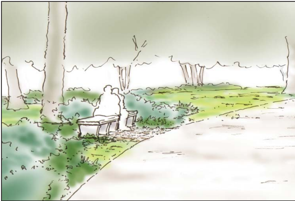
Setting benches a short distance off of the path edge would make them less attainable and attractive to skateboarders. Setting them off the path with a backdrop of plantings would be following one of J.F. Dawson's (Olmsted Brothers) original suggestions.
